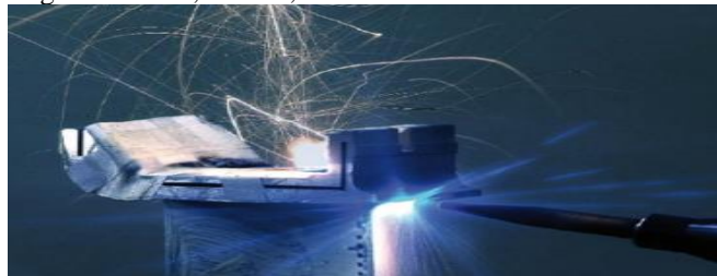
Figure 5: Turbine blade during laser drilling
