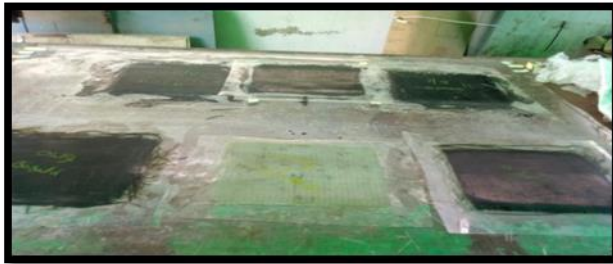
Figure 27 before cutting the specimen (curing period)
