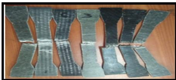
Figure 40 tensile strength materials specimens
