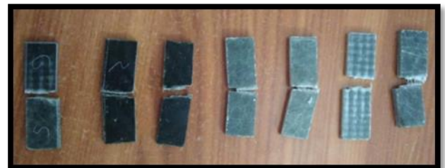
Figure 42 impact strength specimens of all materials
