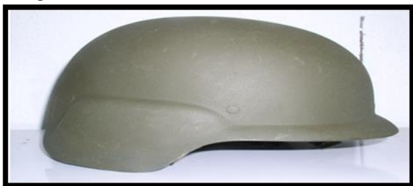
Figure 12 Light weight natural composites military Helmet
