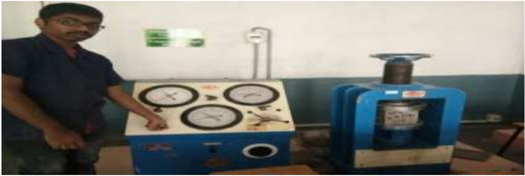
Figure 7 compression test for 30% of foundry sand
