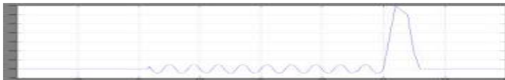
Fig.3.11 Short-circuiting PV panels dc-link voltage when applying a 60% SLG voltages sag at MV side of the transformer
