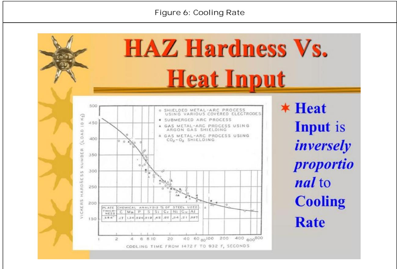
★ Heat Input is inversely proportional to Cooling Rate
