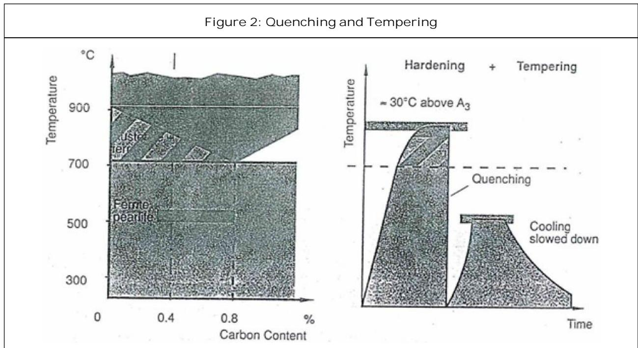
the hardening process, it is possible to increase the ductility of the structure to the same extent as its hardness decreases. Both characteristics are directly coupled with each other and are directly dependent on the temperature.
