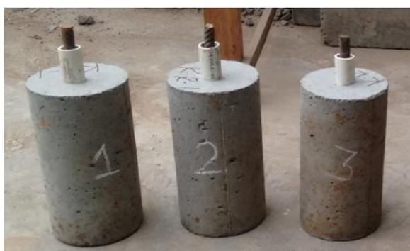
casted for flexural strength. Similarly fifteen cylindrical specimens of size 100 mm diameter and 200 mm length are casted for split tensile strength and young's modulus. To evaluate the corrosion resistance, the specimens with the following nomenclature are casted as shown in Figure 2. A bar diameter 16 mm and length 35 cm. The bar kept with a clear cover 40 mm on bottom for the cylinder specimen. The cylinder specimen size is 150 mm dia and 300 mm height.
