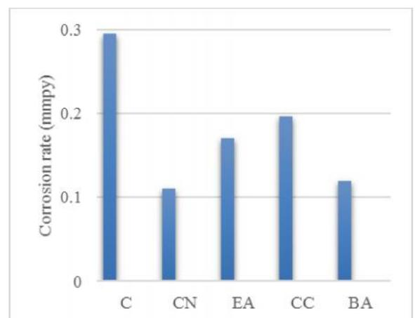
concrete. The high electron's movement results in the increase in current rate. The green corrosion inhibitors are showed better results compared to conventional concrete.
